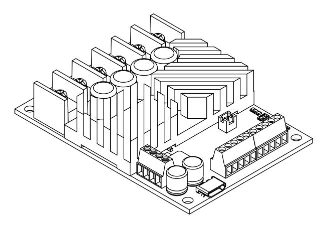
RoboClaw ST 2x45A, 34VDC Dual Channel Brushed DC Motor Controller
